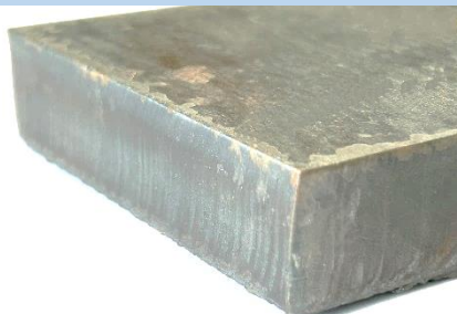
20mm steel cut with Pi 701 pro 70A - 520mm/min
